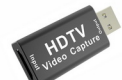
DD601 USB 2.0 HDMI Capture Card HDMI resolution: Max input can be 4K@30Hz Video output resolution: Max output can be 1080P@30Hz Support video format: 8/10/12bit deep color cable distance: <math>\leq 15m</math> AWG26 HDMI standard cable
